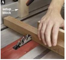
Butt the workpiece against the setup block, holding it securely against the miter gauge. Then make the first cut.
