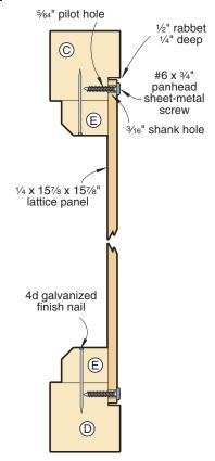
dadoes facing up. This will be the back side. Lay the short uprights (B) just outside the long uprights. Now spread an exterior-grade glue in the dadoes. Join the long and short crossbars to the uprights with the dadoes facing down to lock the pieces together. Using the shank holes in the crossbars as guides, drill  $\frac{3}{32"}$ pilot holes into the uprights. Then secure each joint with a  $1\frac{1}{4}$ " deck screw.
